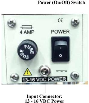
Input Connector: 13 - 16 VDC Power Inlet / Emergency Disconnect Device
